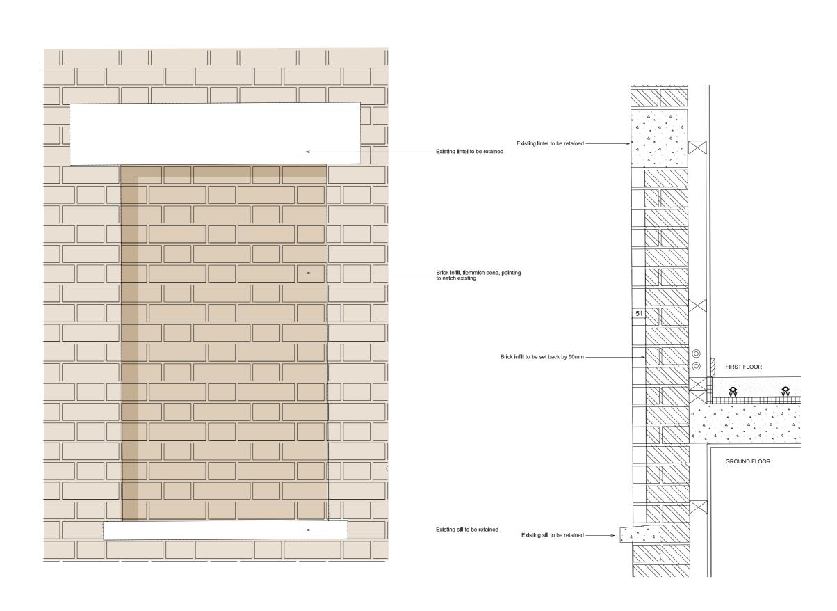
01 Elevation 1:10@ A3 02 Section through infilled opening 1:10@ A3
