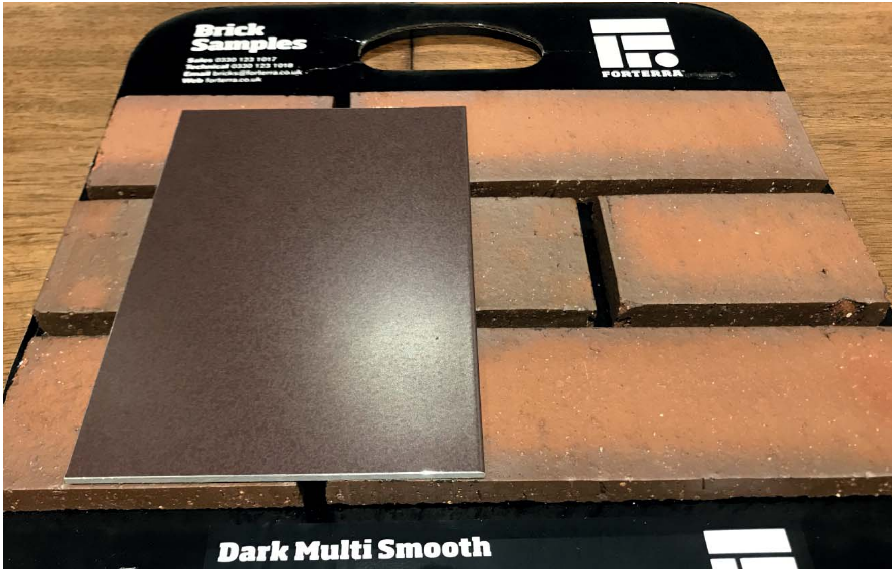
Photograph of red metal cladding taken on site shown next to the brick sample matched with the existing brickwork.
