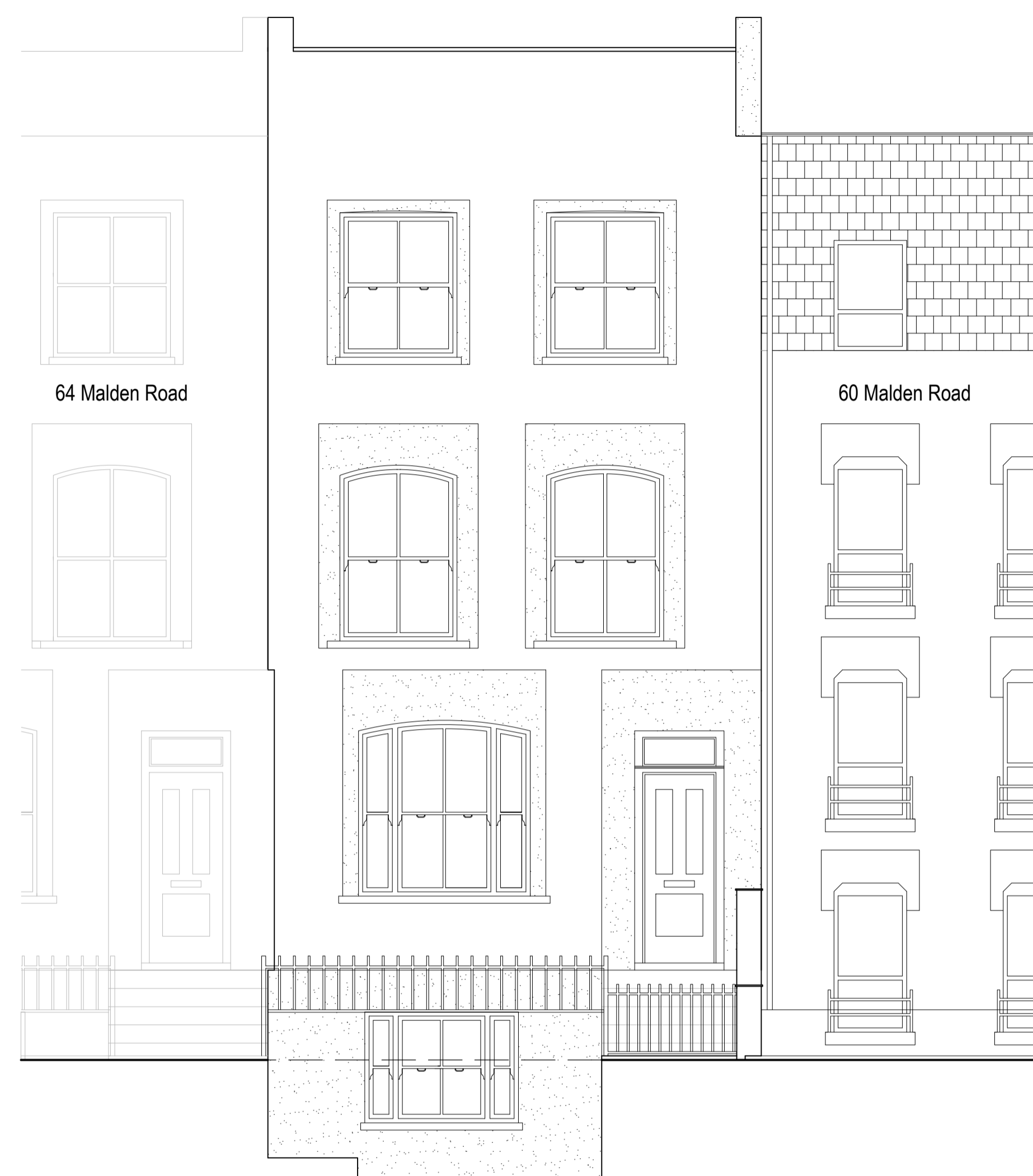
Proposed Front Elevation (West) - 1:50@A1
