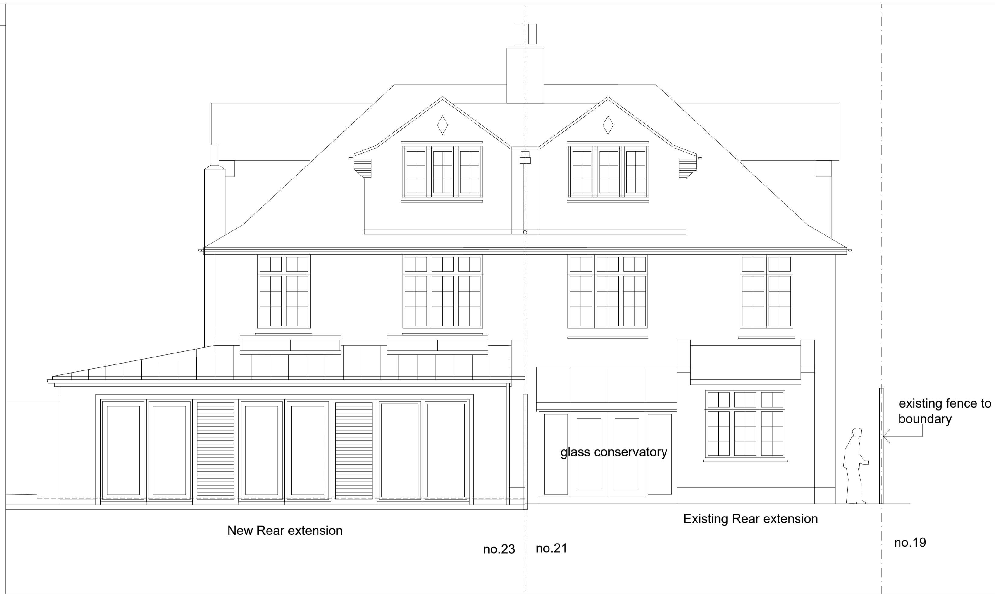
REAR GARDEN NORTH ELEVATION no.21
