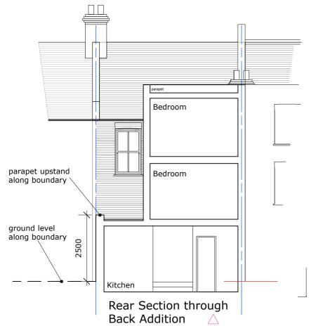
Rev. A: 05.07.17 Height of flank wall along boundary reduced to 2.5m.
