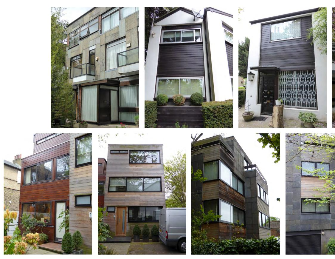
The images on this sheet show the glazing and fenestration variability within the immediate mews area. The proposals to 6 Oak Hill Park Mews seek to replicate the powder coated aluminum detailing found on the existing buildings within the mews with small profile detailing to the front façade, which has the most prominence to the public realm.
