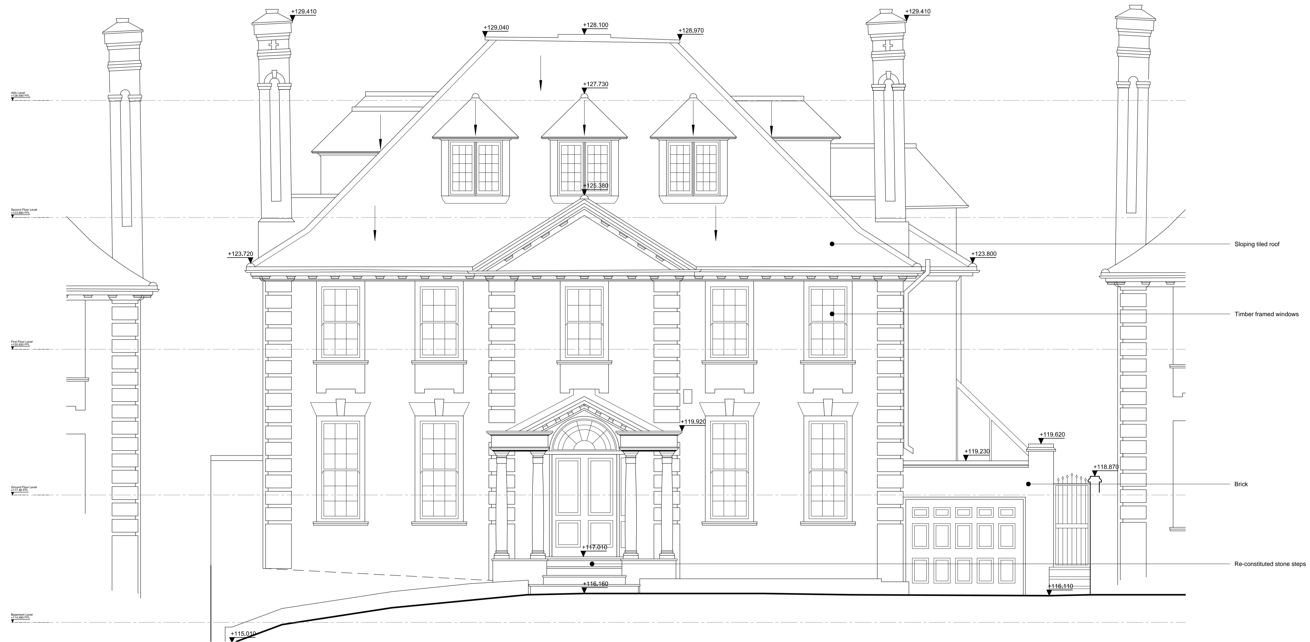
01 Proposed Front Elevation - A D3700 SCALE: 1:50
