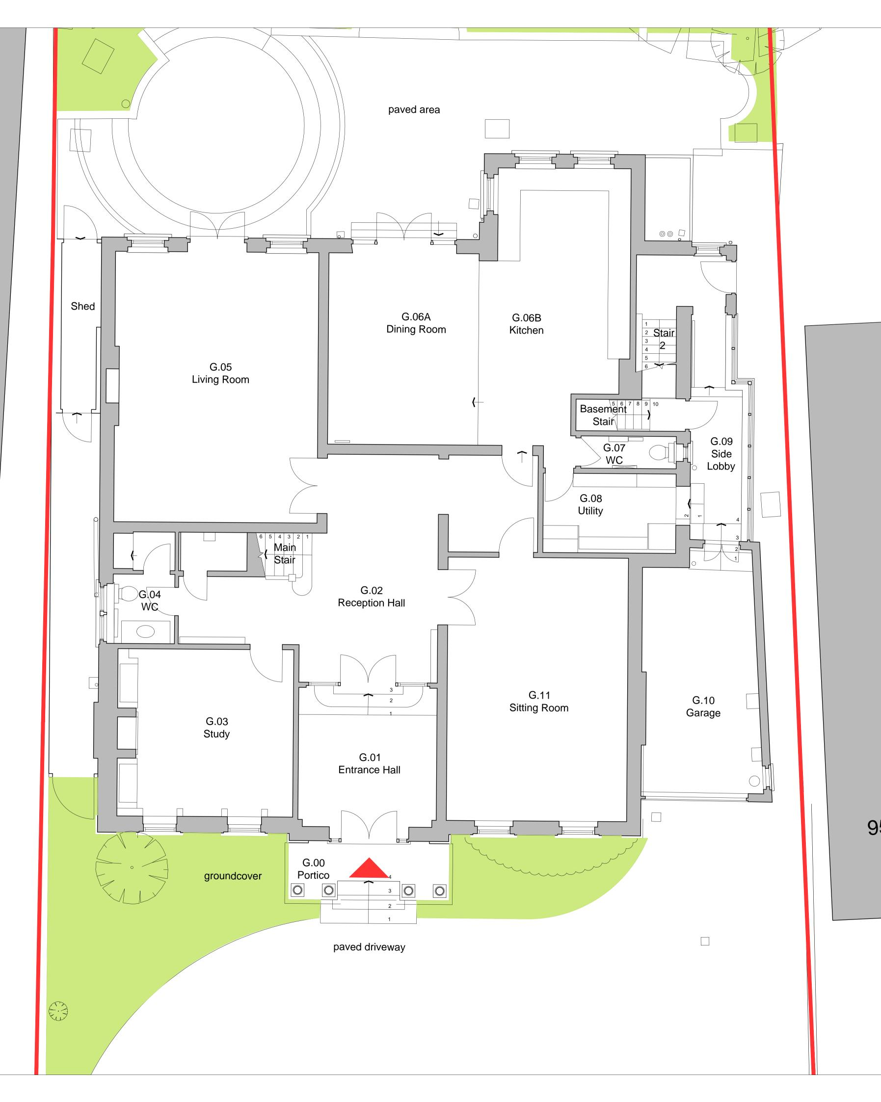
01 Existing Plan - Ground Floor D(0)1100 SCALE: 1:50
