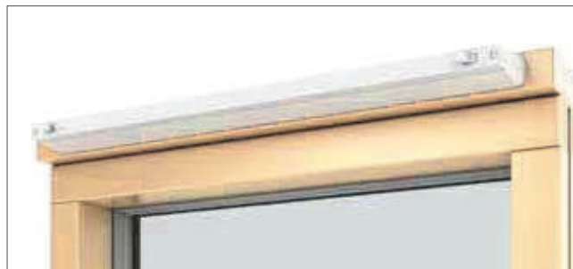
Acoustic trickle vent. The vent is machined into a timber packer with an external aluminium profile in the same colour as the window sashes. Documentation on air flow can be requested. Achieves a sound reduction value of D_{n,e,w} 40 dB.
