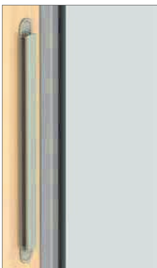
Click vent. Anodized surface finish. Fully concealed. Free ventilation opening in elements with 24mm glazing: 4000mm². Free ventilation opening in elements with 48mm glazing: 3000mm².
