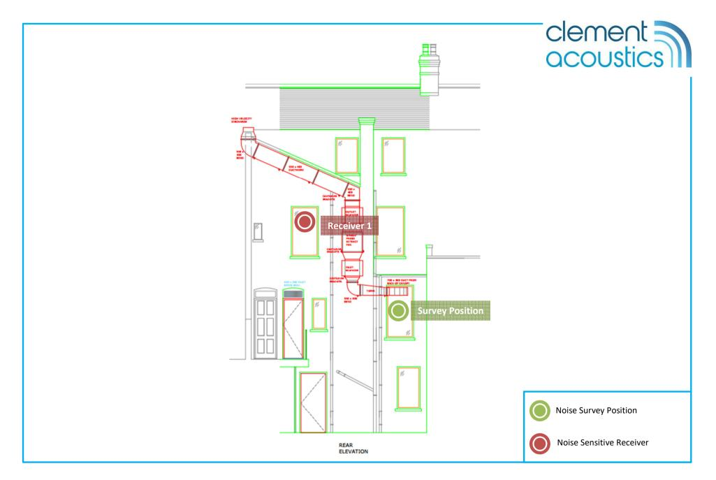
**12408-SP1** Indicative site plan indicating noise monitoring position and nearest noise sensitive receiver
