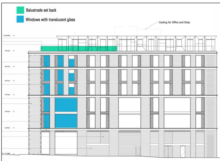
Figure 9 (left): Level of translucent glass on the side elevation of Building 1 which faces Linton House. Windows on the upper floors that are opposite habitable rooms would be obscured and fixed shut below 1.7m.
