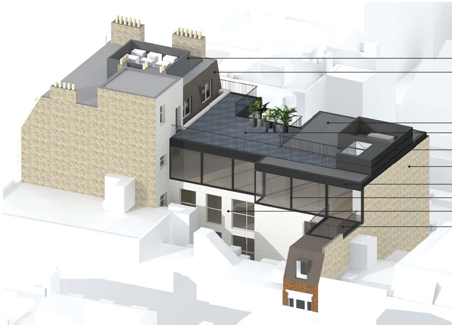
Axo view from rear of building showing new materials at 3rd floor office, 4th floor terrace and 5th floor roof plant.
