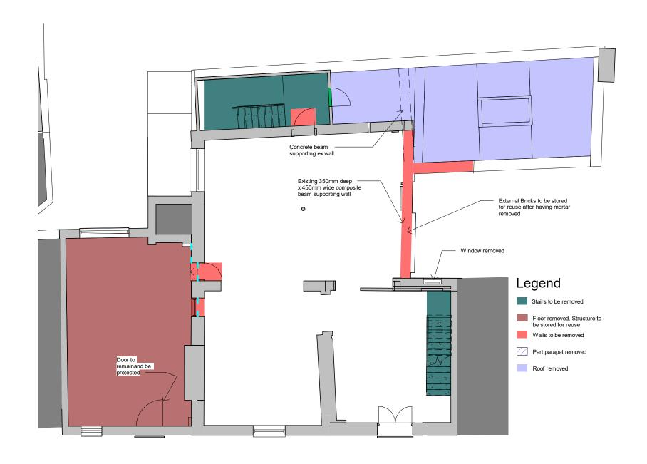
This drawing must be read in conjunction with demolition specification MID/xx/xxx.
