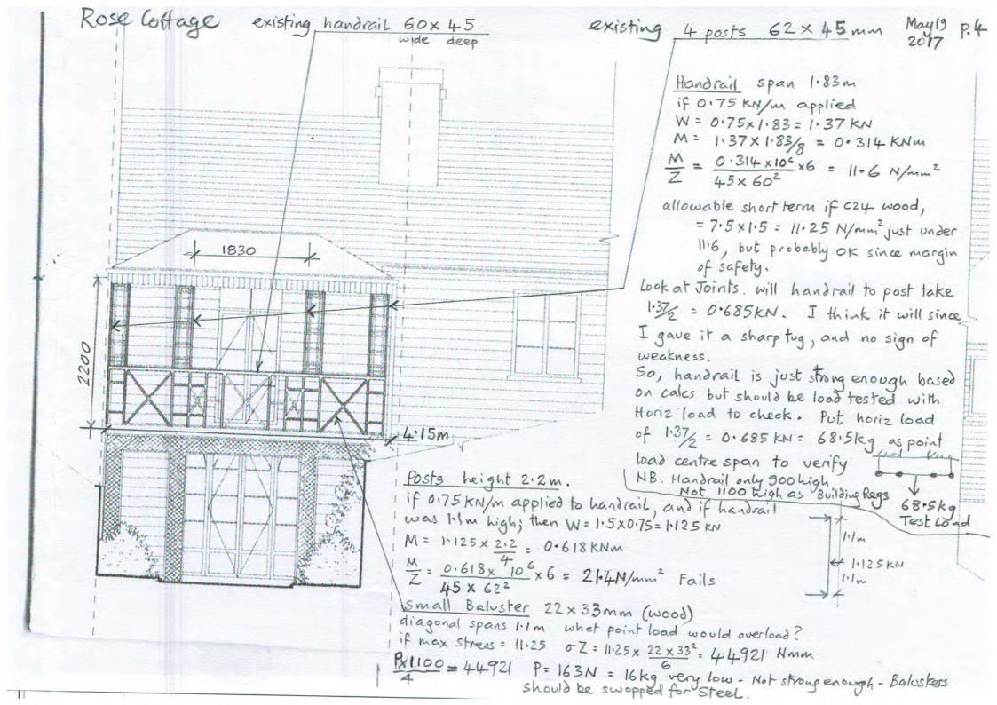
New 25x25 steel handrail white at 1100 ábove deck
