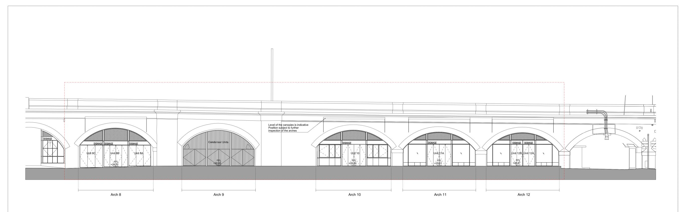
O1 Proposed North Elevation - Arches 8 to 12 SCALE 1:100
