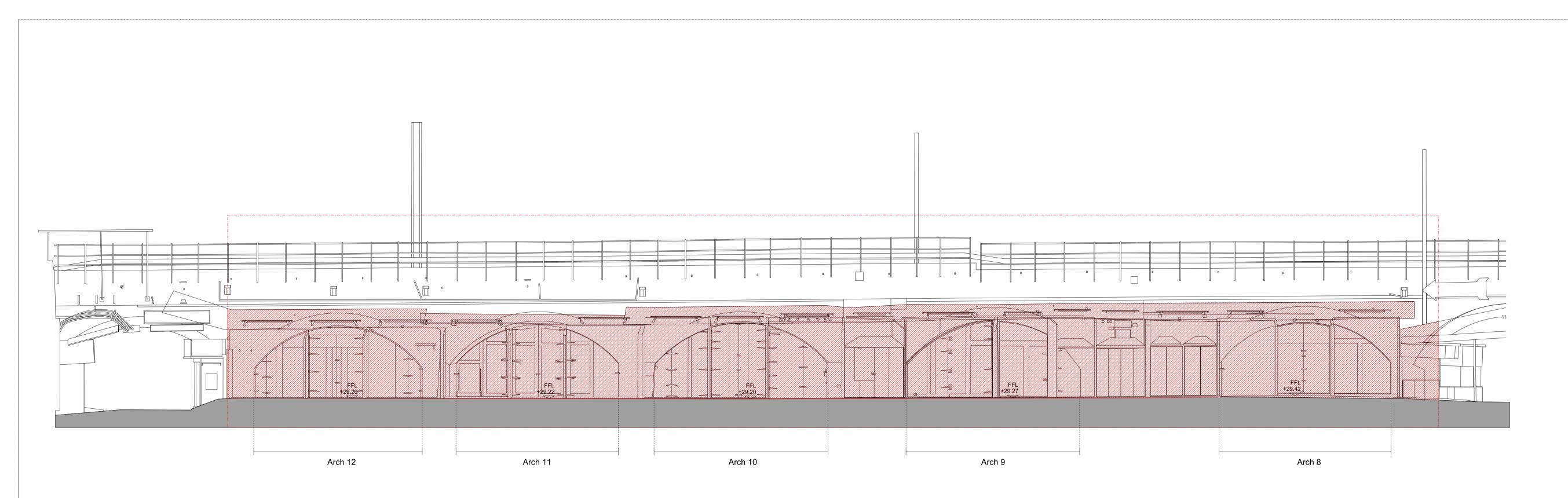
O1 South Elevation Demolition Scope - Arches 8 to 12 SCALE 1:100
