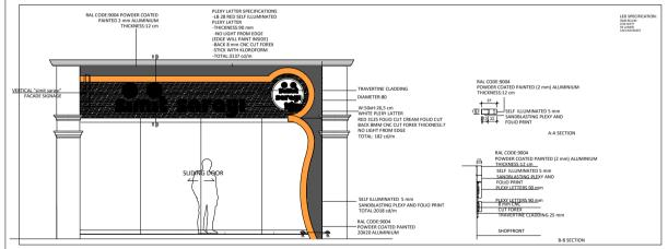
AS BUILT SIGNAGE DETAIL ELEVATION
