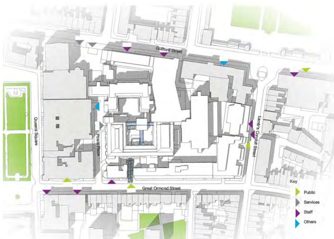
Figure 9: Plan showing the entrances for the public (in green), services (in grey), staff (in purple) and other (in blue) and internal hospital corridors, edged in light blue that links the Variety Club Building to the Frontage Building at Levels 2 and 3.
