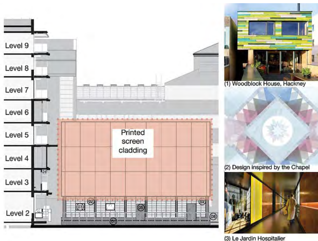
Figure 11: (Left) North Elevation showing the printed screen cladding panel as seen from the courtyard and (right) examples of printed cladding from GOSH Arts shortlist of Artists
