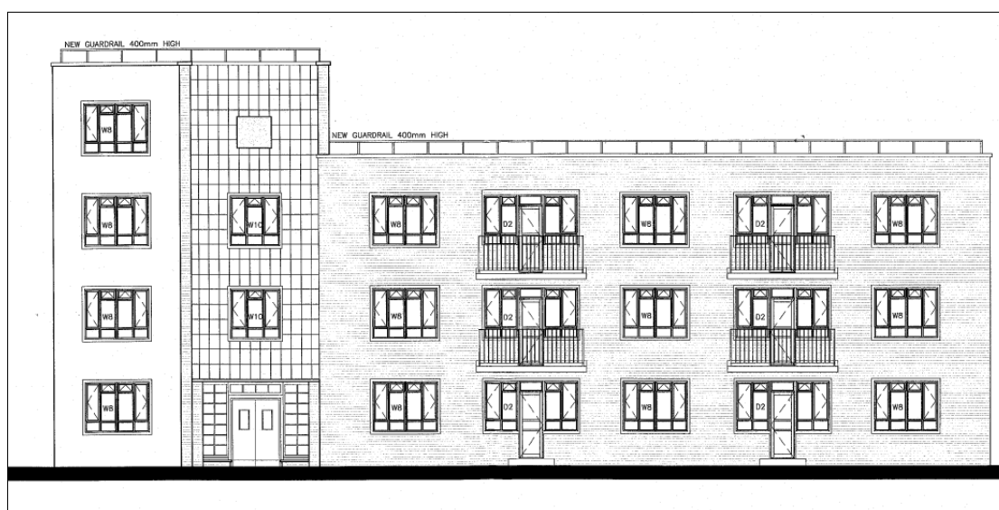
Figure 7: Extract from the permitted, submitted drawings for replacement doors windows and installation of guardrails round rooftop of Troyes House.
