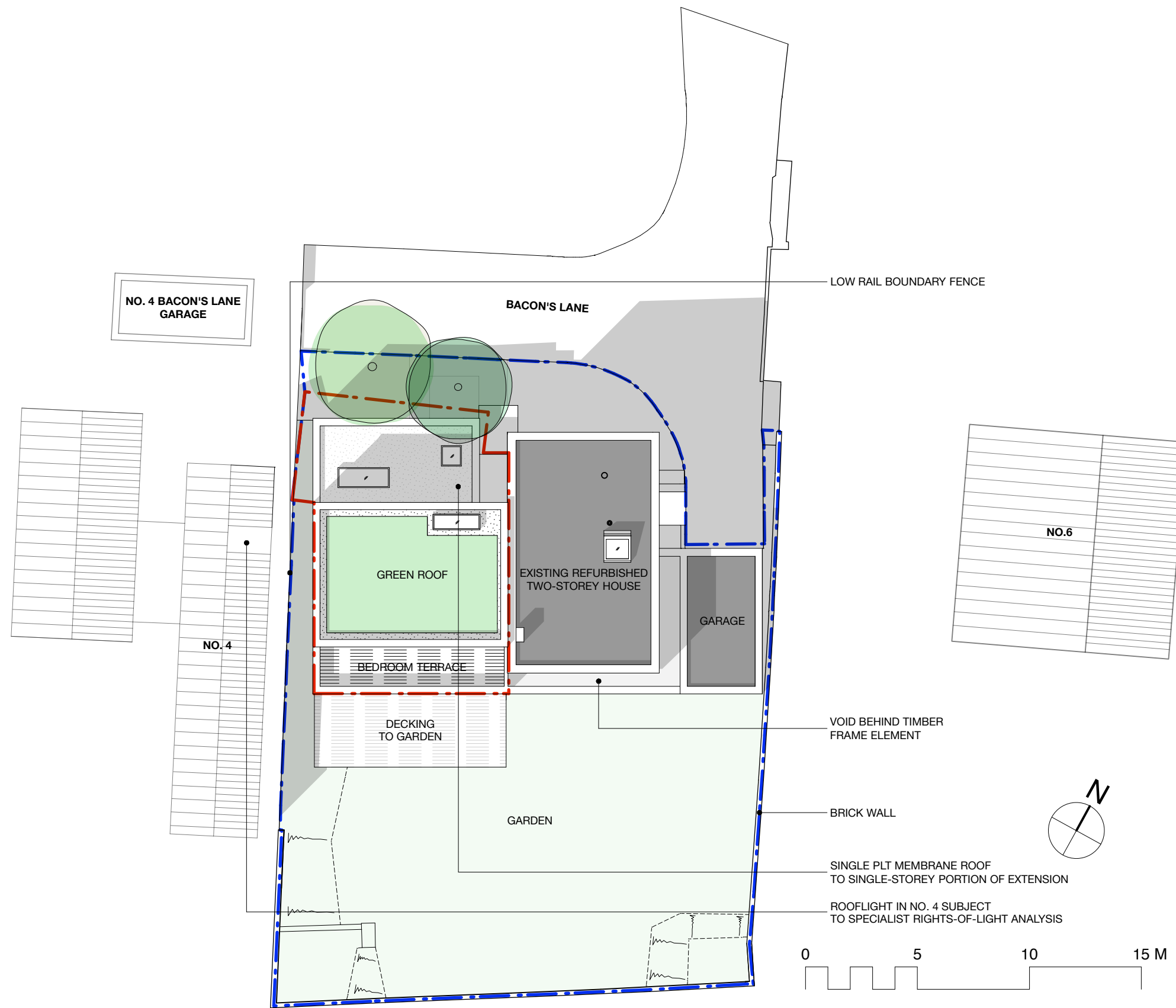
01 PROPOSED LAYOUT & ROOF PLAN 1:200
