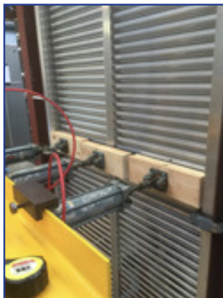
Horizontal Line Load (Internal view of test)
