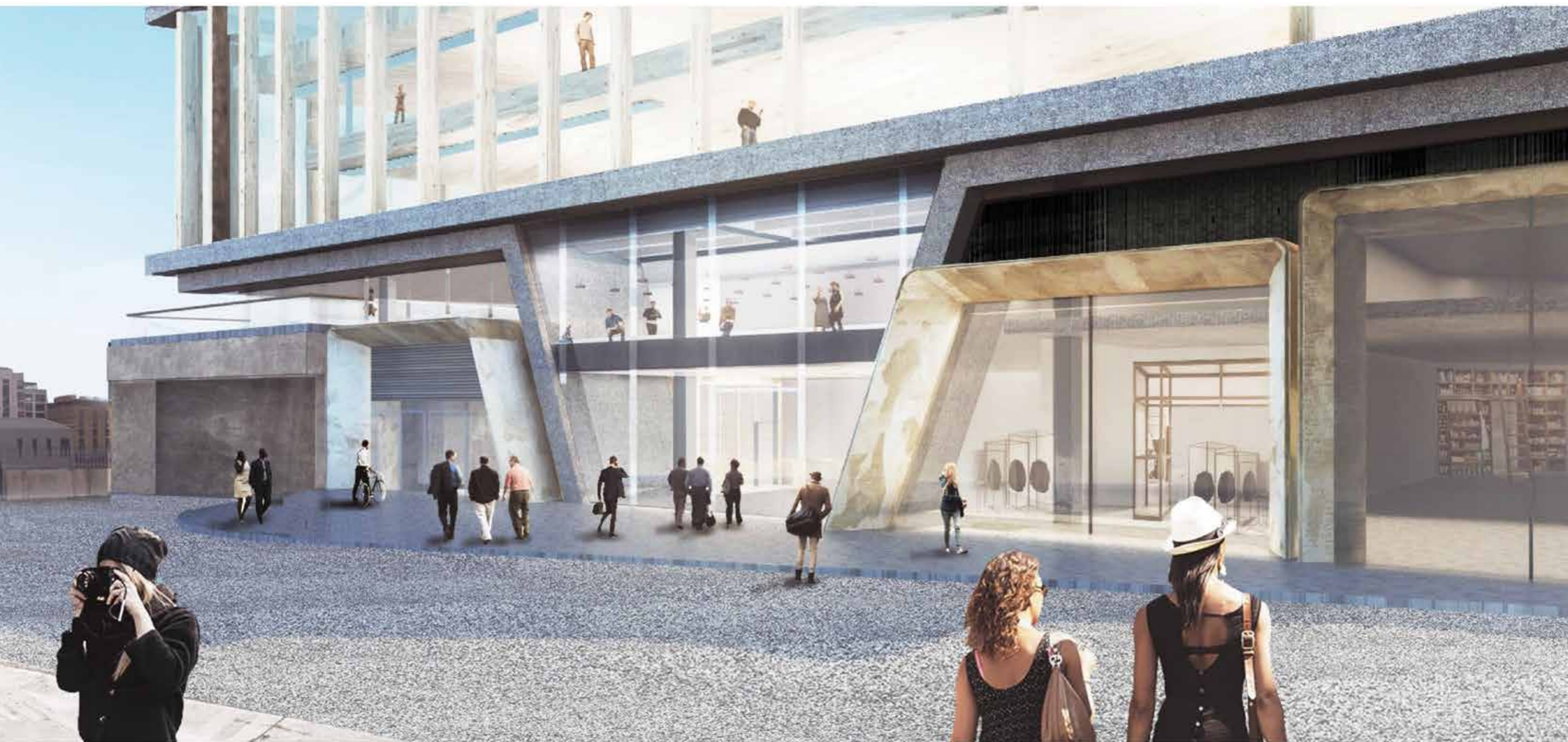
Figure 134: Illustrative view of the entrances on the north facade, comprising from left to right: the Access Ramp, the cycle store entrance, the North Entrance and the North Anchor retail unit
