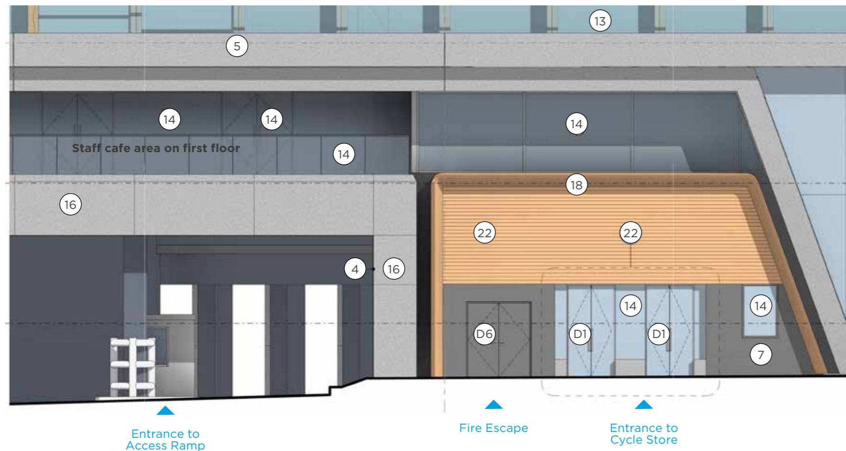
Figure 110: Elevation drawing showing the materials proposed for the entrances on the northern facade of the building
