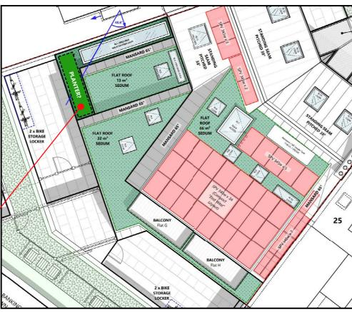
The 2nd floor roof already takes the weight of 29 solar panels and the rainwater harvesting header tank, with minimal space for planting.
