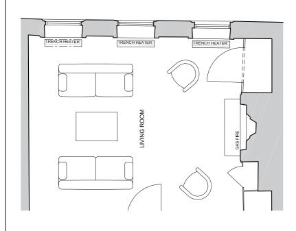
04 - TRENCH HEATES LOCATED BELOW WINDOWS - SECOND AND THIRD FLOOR ONLY (PLAN SHOWING SECOND FLOOR FRONT WINDOWS)
