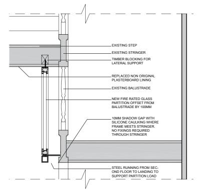
04 - STAIR SECTION THROUGH SEPARATING WALL - PROPOSED
