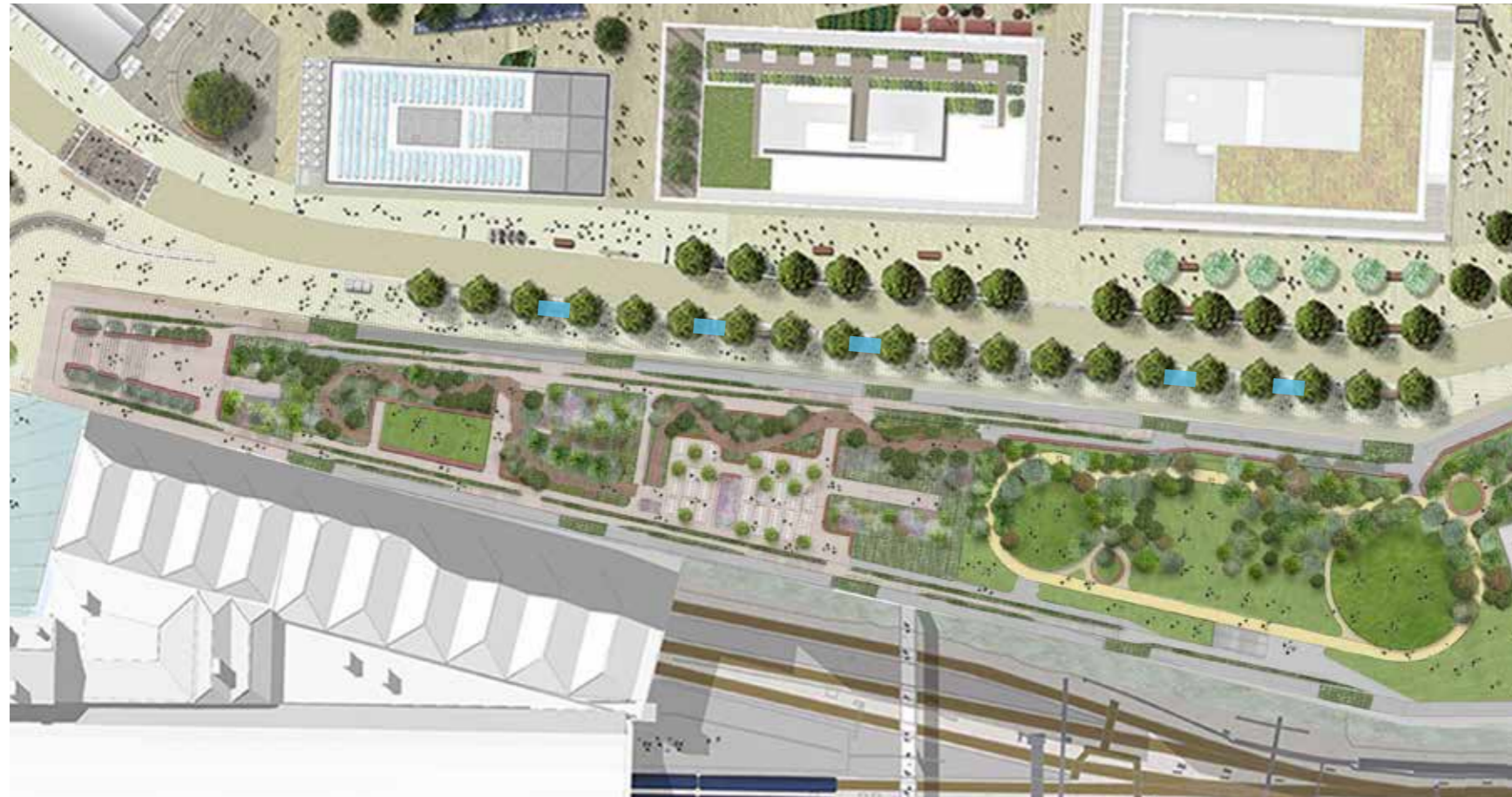
Figure 65: Proposed visitor and retail cycle parking within public realm, shown in blue, each with 5 racks (10 spaces)
