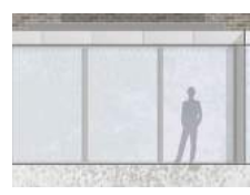
Window Frames - Light Natural Aluminium which will also line the column in the centre.
