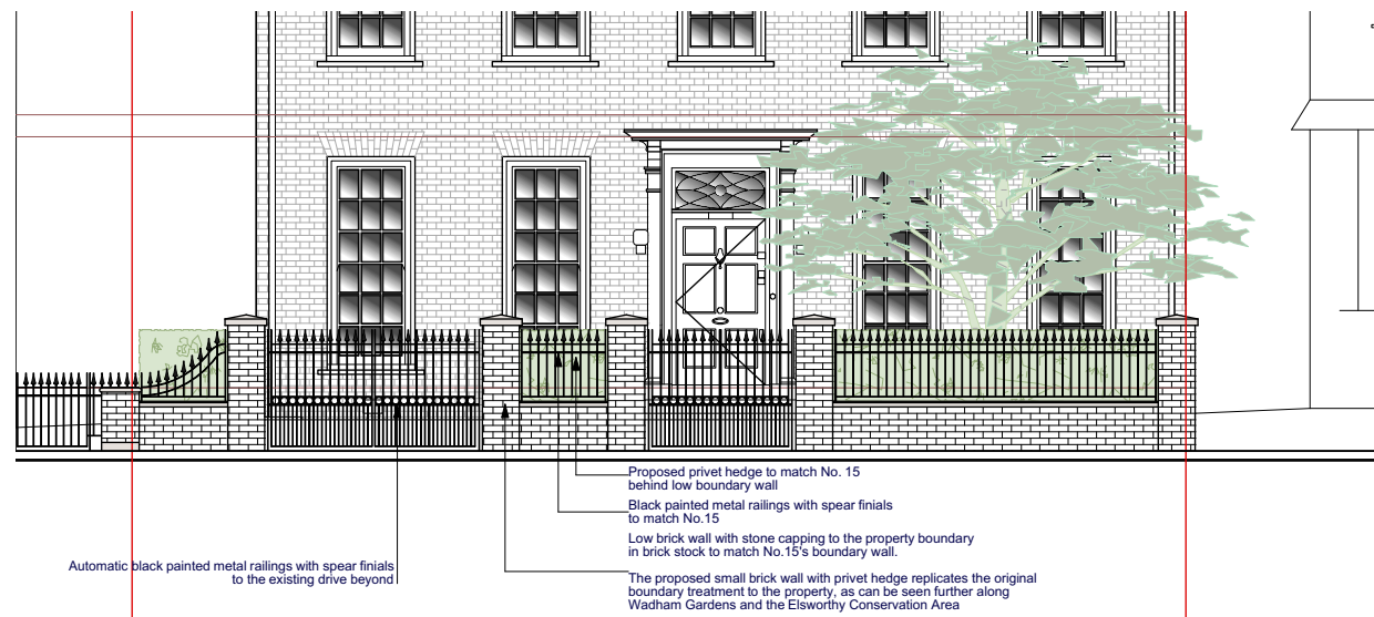
ELEVATION OF FRONT BOUNDARY AS PER PLANNING PERMISSION APPROVED DRAWING 462-GA.16 SCALE 1:100
