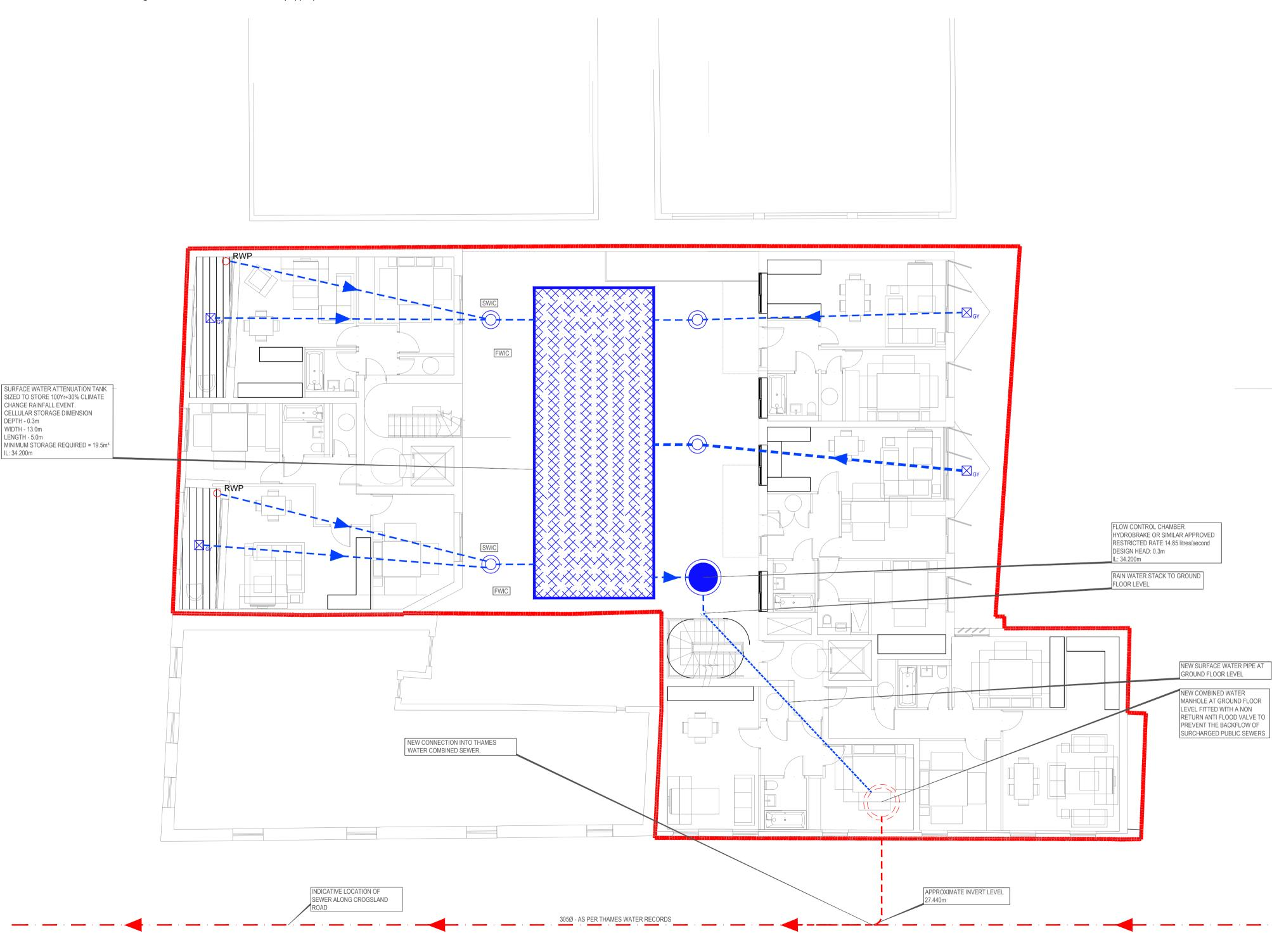
All drainage connecting to the public sewer network shall not commence until receipt of the approval from the drainage authority and shall comply with requirements using vitrified clay pipework to BS EN 295 with plain sleeved or socketed flexible joints subject to their approval.
