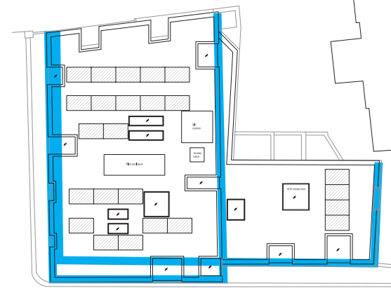
Location of acoustically enhanced facades (for full details refer to the acoustic report)
