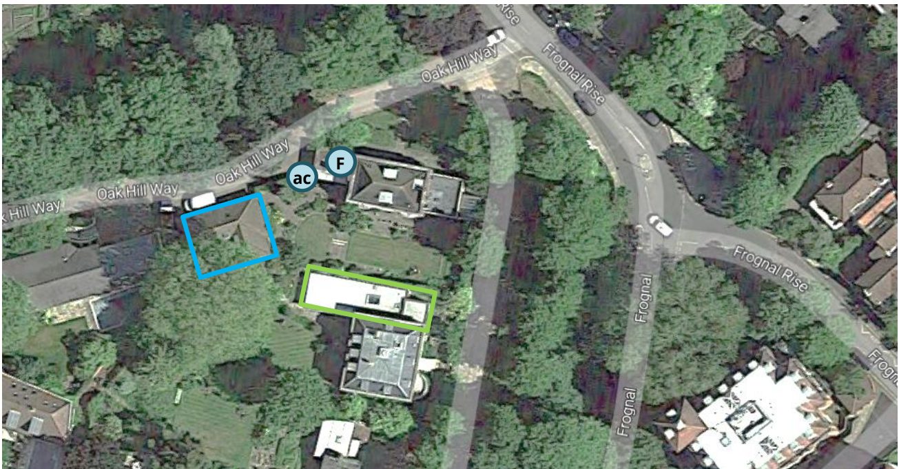
Figure 2.1: Site location, with the position of the fixed microphone (F) and the nearest receptors (in green and blue) and the position of the air conditioning units (ac)
