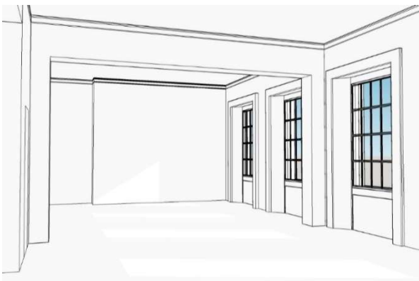
Proposed removal of chimney breast. The downstand is retained to clearly mark the historic division of the rooms, with existing cornice retained, and pieced in where necessary.
