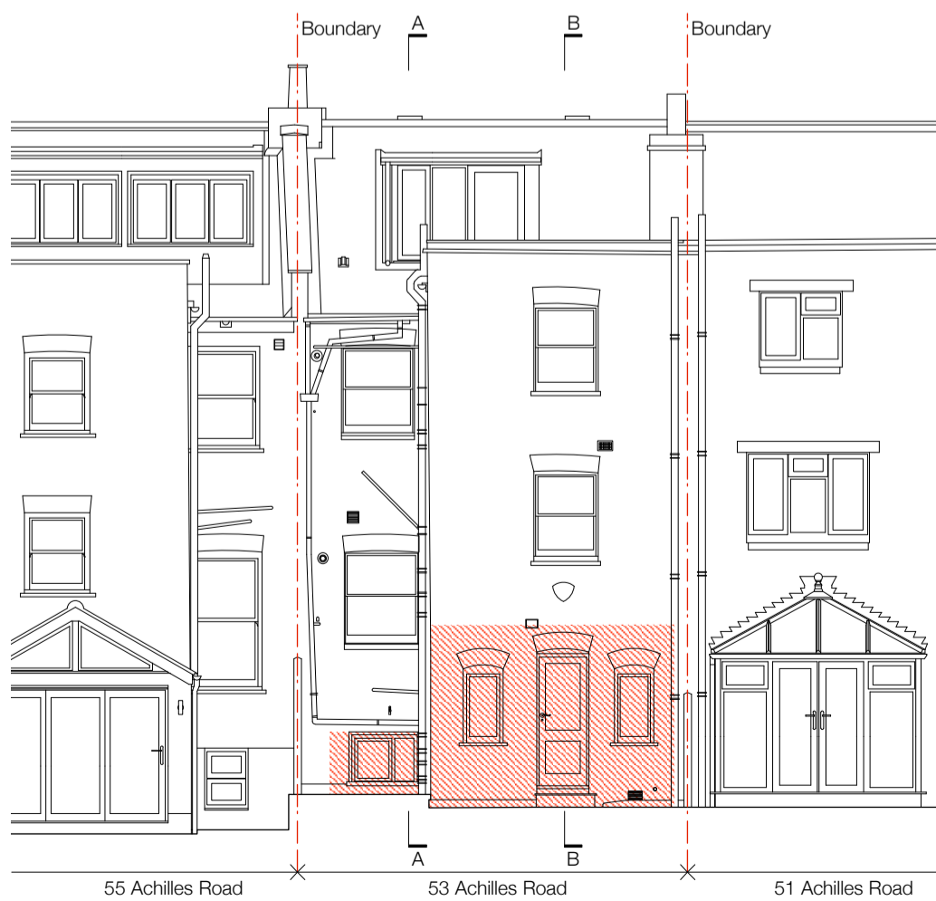
REAR ELEVATION DEMOLITION
