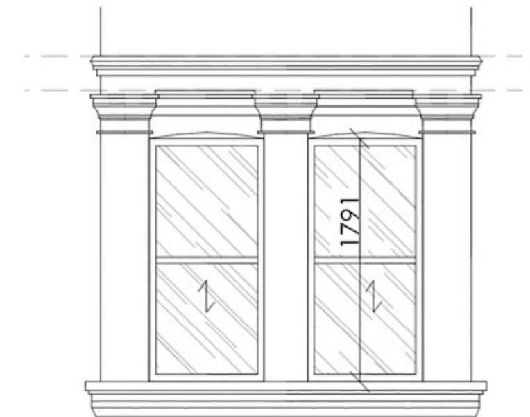
Existing front window elevation
