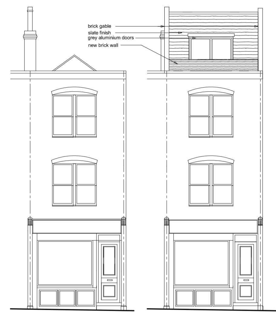
FRONT ELEVATION (EXISTING)
