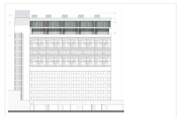
The proposed upward extension of the main residential tower will create five 3 bed, dual aspect duplex units, each with its own roof garden. This will be of a steel frame construction on padstones inline with the existing structural supports. The existing scaffold will be extended upwards by 8m with a temporary roof extending over the building
