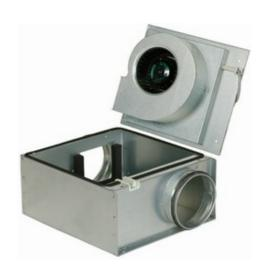
The KVO EC 100-160 models have a single-inlet centrifugal fan with forward-curved blades and a maintenance-free external rotor motor(EC). KVO EC 200-315 models have a single-inlet centrifugal fan with backward-curved blades and a maintenance-free external rotor motor(EC). These fans develop relatively high static pressure and have a very high efficiency. The fans are delivered with a pre-wired potentiometer (0-10V) that allows you to easily find the desired working point.
