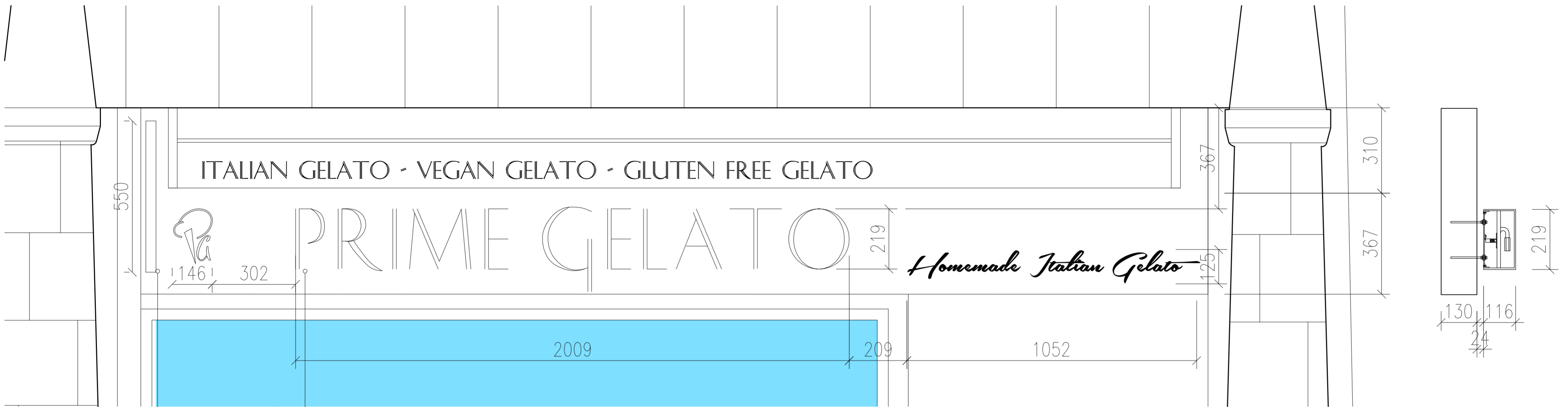
INTERNALLY ILLUMINATED SIGN SCALE 1:10 @ A2
