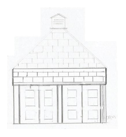
New Bin room to be brick construction on 1mtr deep Strip footing isolated from existing. Bricks to be Yellow London Stock.
