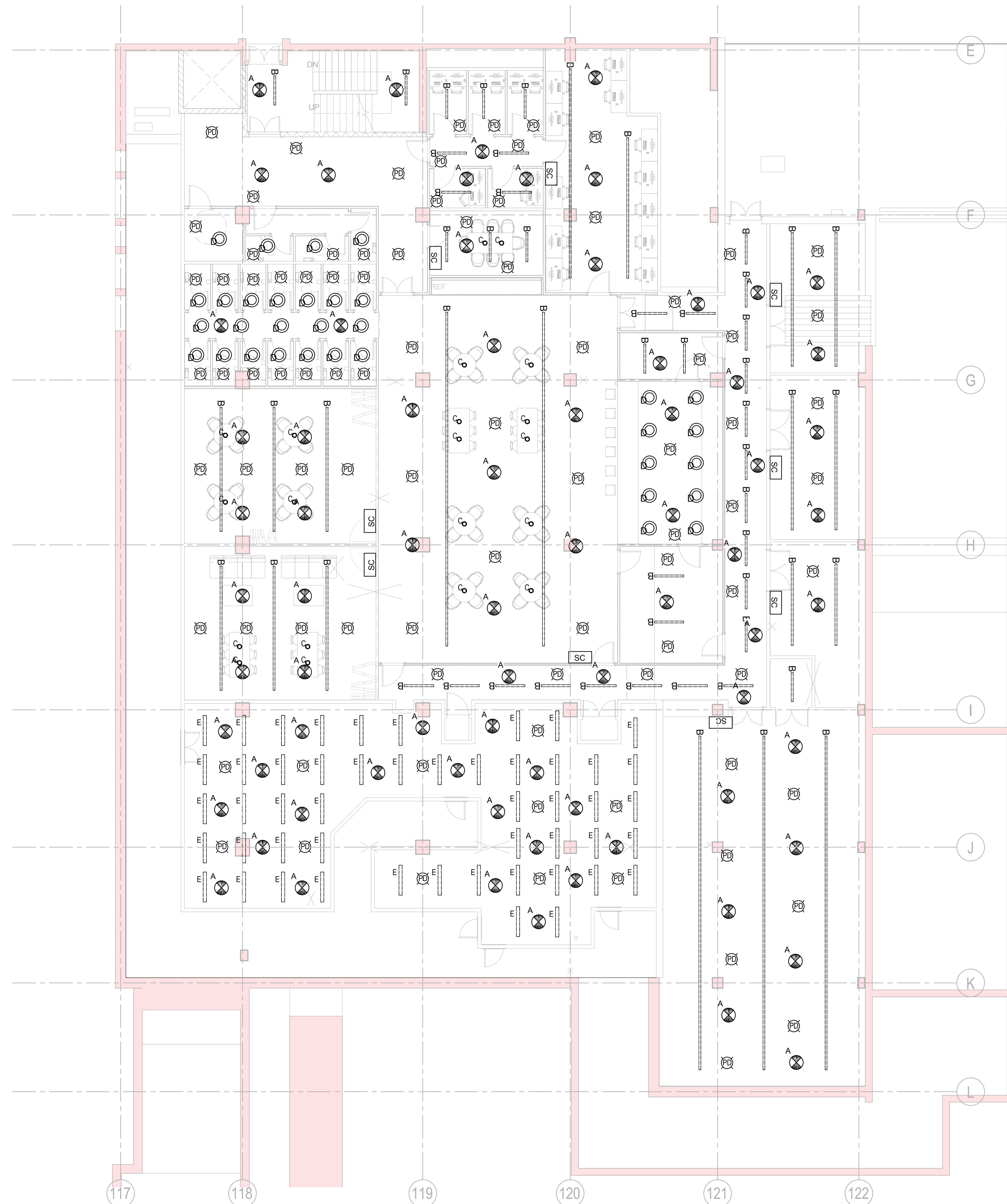
1 Electrical Services Lighting Layout - Level 2 Wing A
