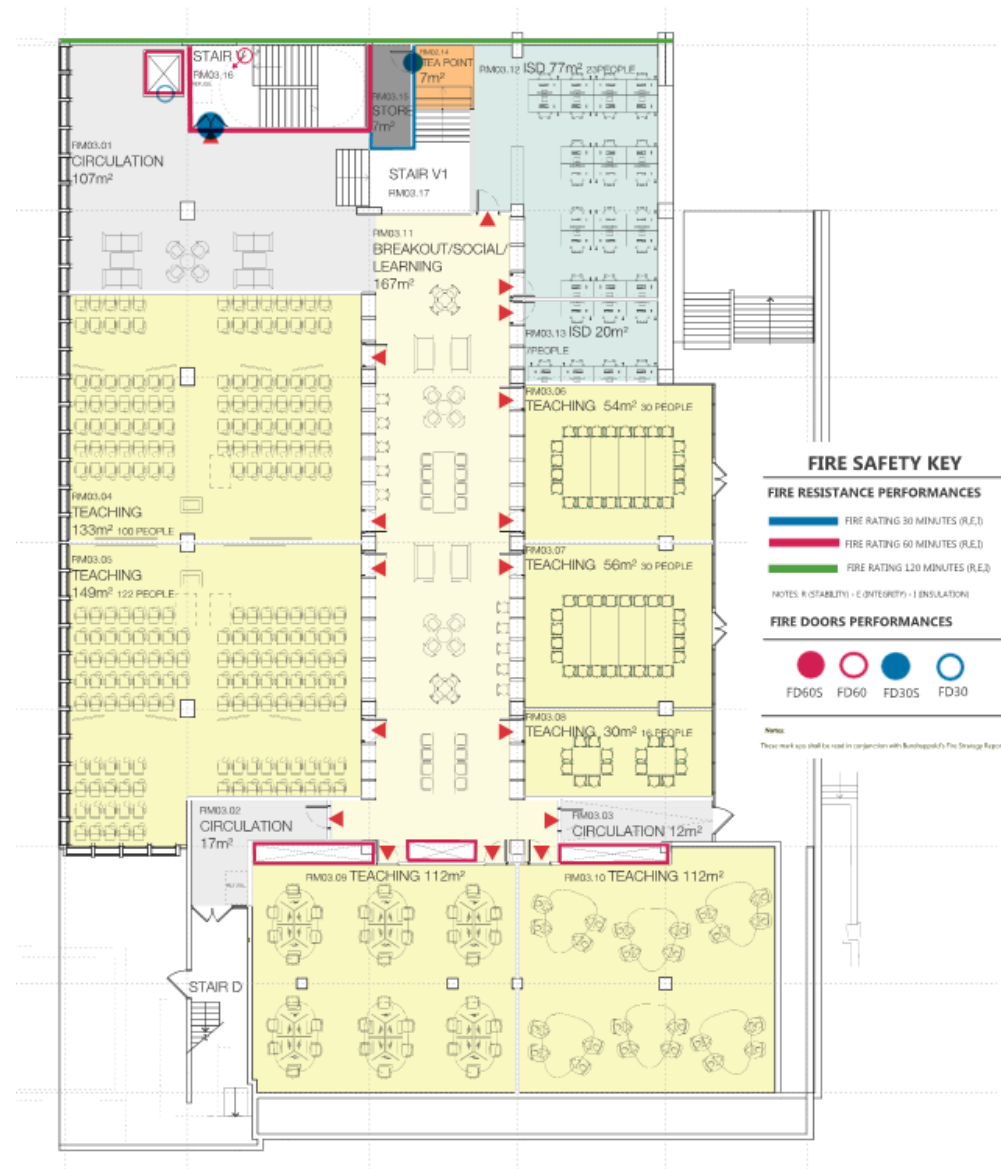
Figure 4—2: Level 03 Wing compartmentation
