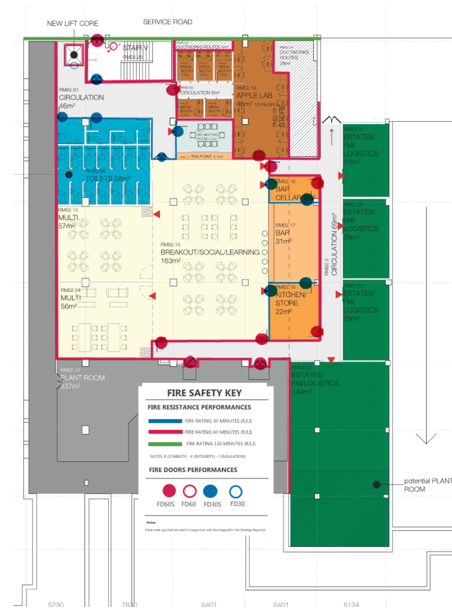
Figure 4—1: Level 02 Wing compartmentation
