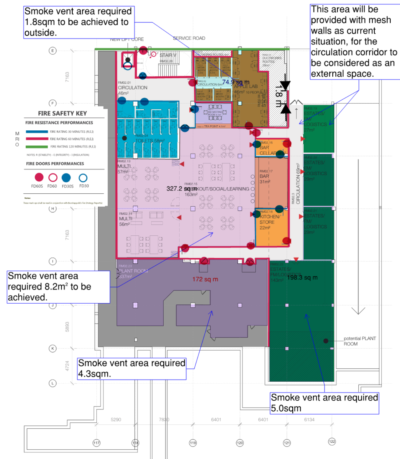
Figure 6—4: Level 02 Wing smoke clearance requirements
