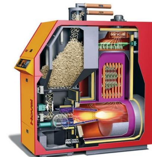
Section of Hopper Fed Biomass Boiler
