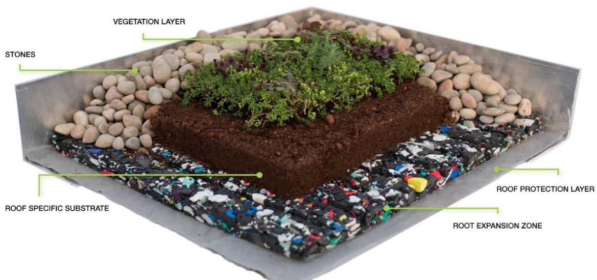
Figure 12: Extensive Sedum Roof Structure
