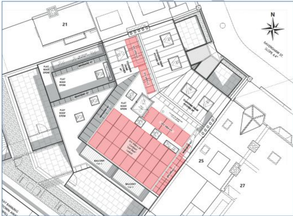
Figure 4: Roof area suitable for installation of Solar PV
