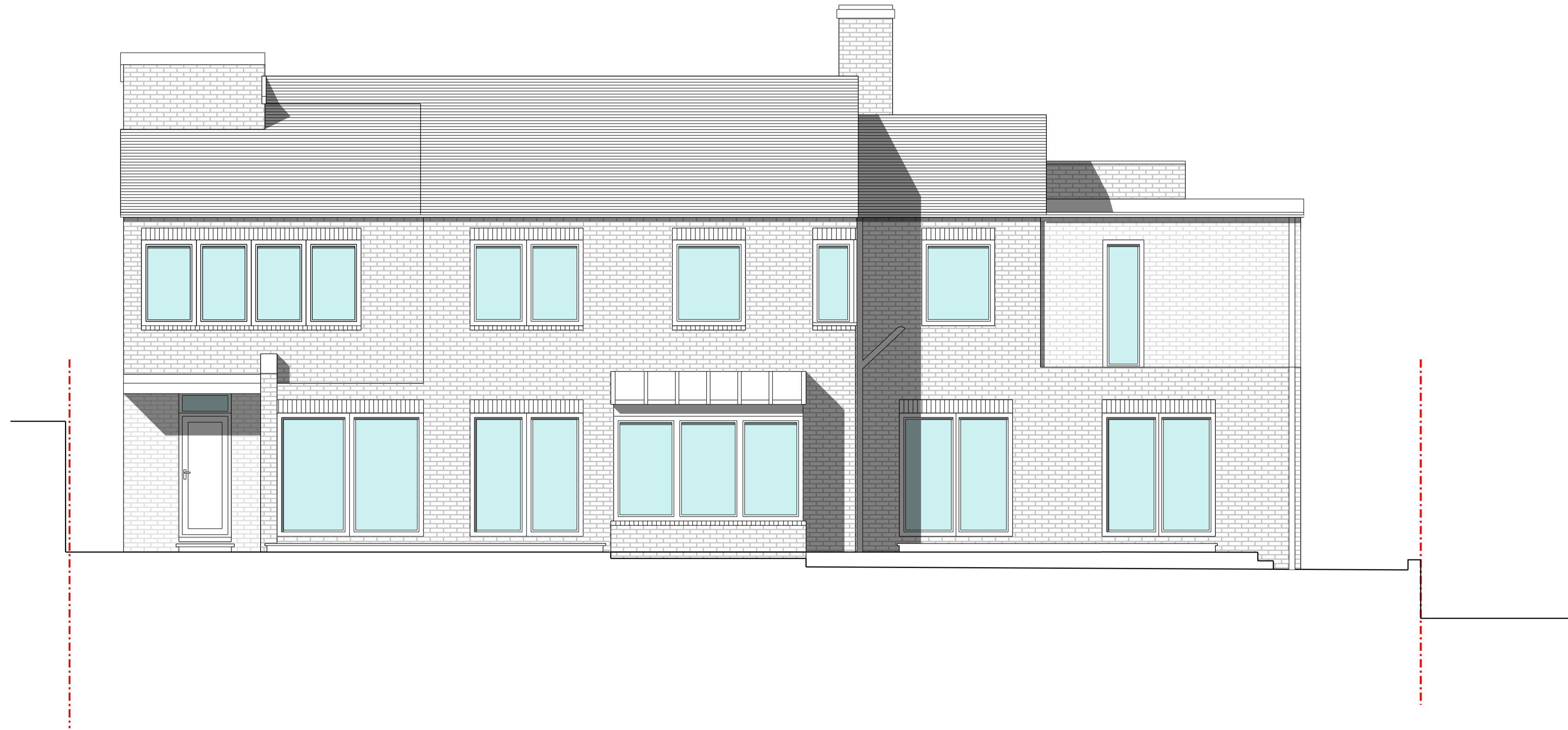
02 REAR (NORTH) ELEVATION AS PROPOSED KAM01_P_131 SCALE 1:50 @ A1
