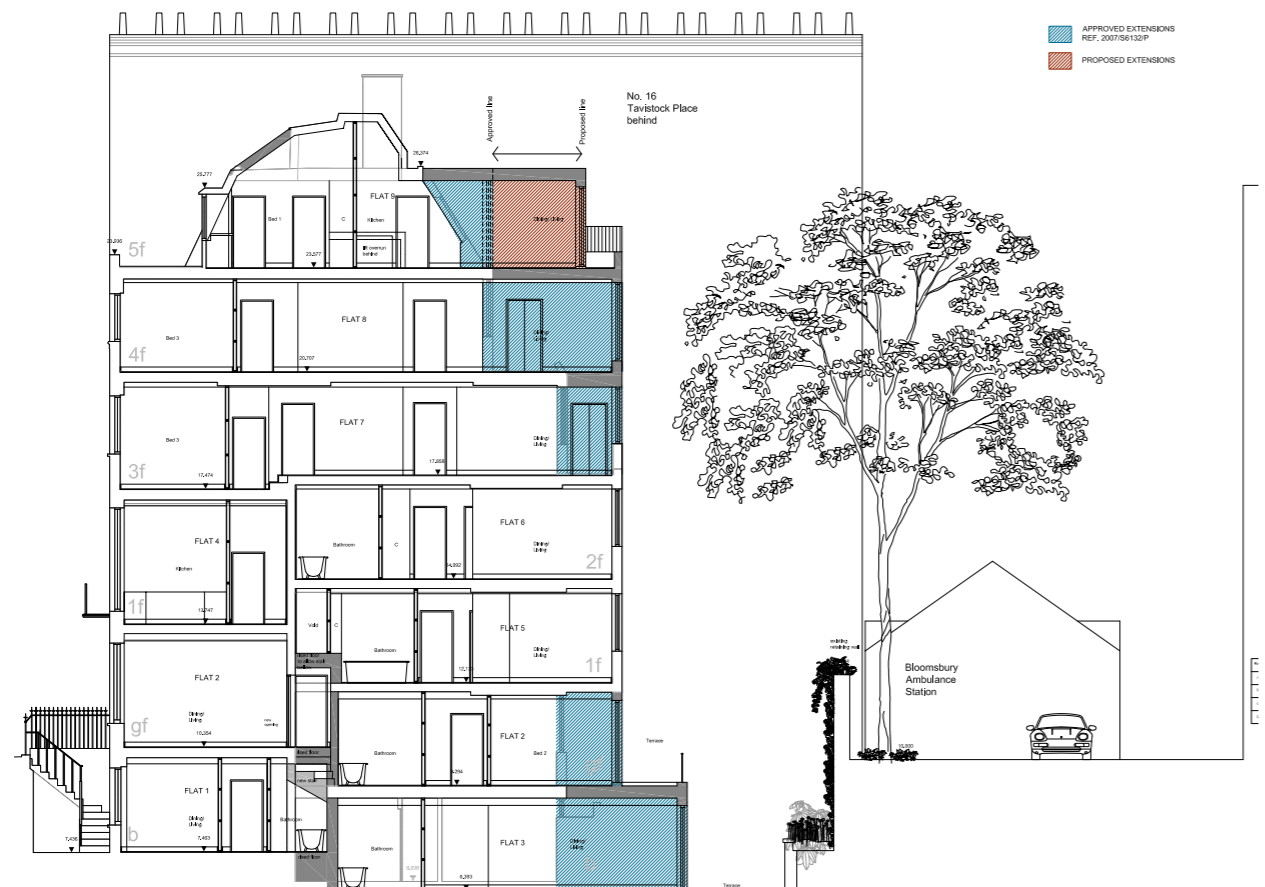
2 Tavistock Place Consented Drawings (ref: 2010/0543/P) Section showing new build extensions in BLUE and RED
