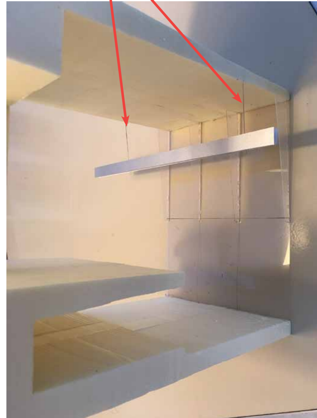
PHOTO OF MODEL SHOWING TROUGH SUSPENSION RODS AT EVERY 4TH FIN (3 GLASS BAYS WIDE).
