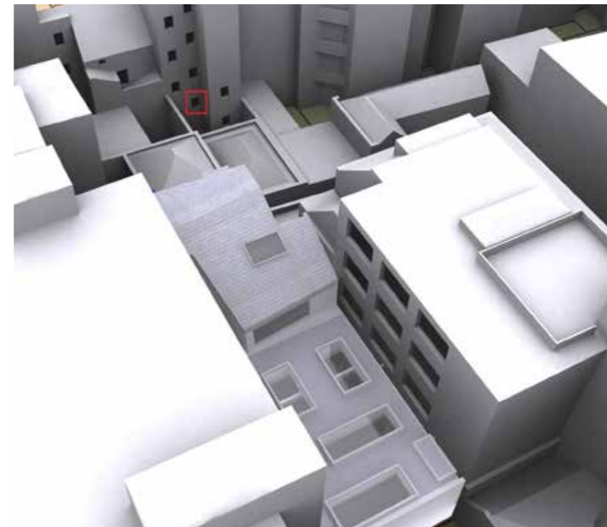
Lighting studies on the originally consented scheme by CHP showing impact on the window
