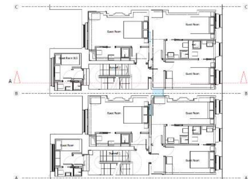
Figure 41: The first floor plan showing blocked up lateral access and opening up of original doorway from landing to rear room.
