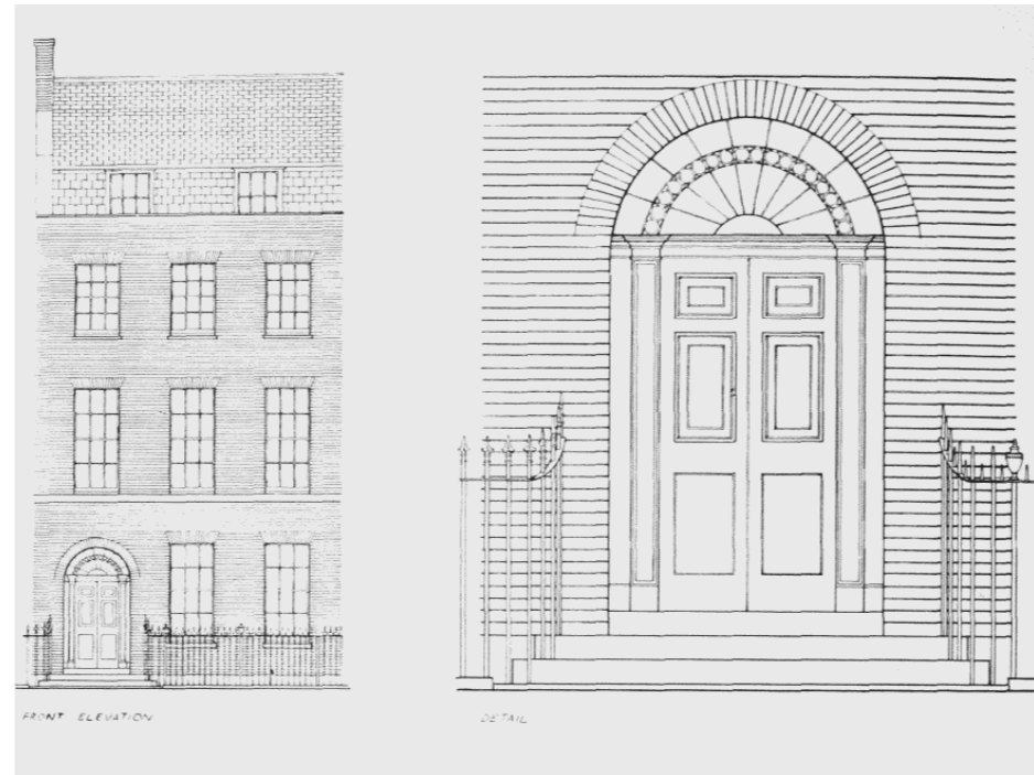
Figure 14: Typical original elevation Gower Street. Notice elaborate fanlight detail no longer extant to either building. Source: Survey of London.
