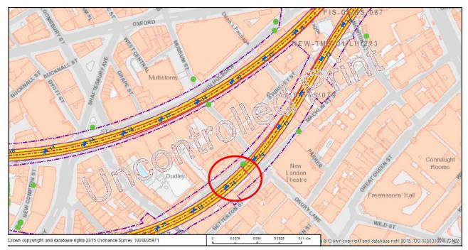
Key: Purple line - Safe-guarded area Yellow area - Tunnel outline Red dotted - Tunnel crown Blue "pins" - Distance between crown and ground level (m)
